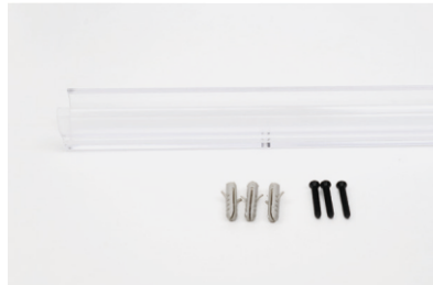
-Name : R25 - Surface mounting with PC profile -Model : R25-IA02 -Attachment: Transparent PC mounting profile, Tapping screws, Expandable rubber plugs Note: Using Transparent PC mounting profile will cause the neon body to compress and stretch, resulting in a dark area at the tail!
